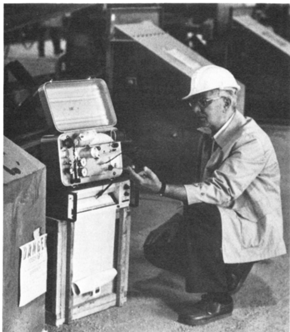
Figure 1. Injecting sample of phosphine into Photovac 10A10 gas chromatograph.
